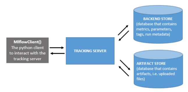
Basically, this schema shows that mlflow separates WHERE the artifacts are logged from HOW they are logged inside your code. You need to setup your mlflow tracking server separately from your code, and then each logging will send a request to the tracking server to store the elements you want to track in the appropriate location. The advantage of such a setup are numerous:
