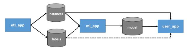
The  $ml\_app$  takes instances (i.e. examples of the business object to handle) as input. This implies that the  $ml\_app$  will include some machine learning-specific preprocessing and not only the model training. It also (optionally) takes labels as inputs if the underlying problem is supervised. Even in this situation, the labels will not be known at inference time so the  $etl\_app$  does not necessarily produce them.
