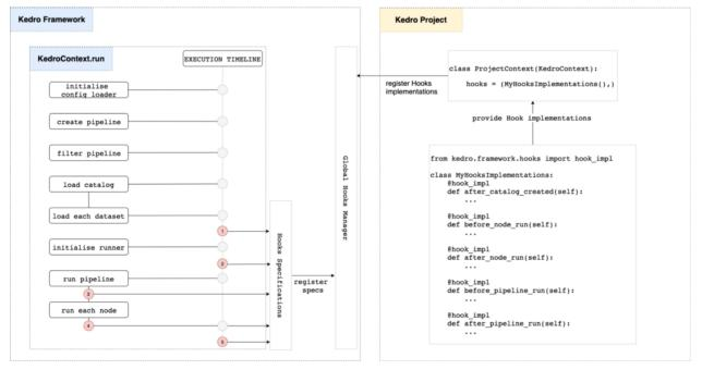
The MlflowNodeHook registers the parameters before each node (entry point number 3 on above picture) by calling mlflow.log\_parameter(param\_name, param\_value) on each parameters of the node.
