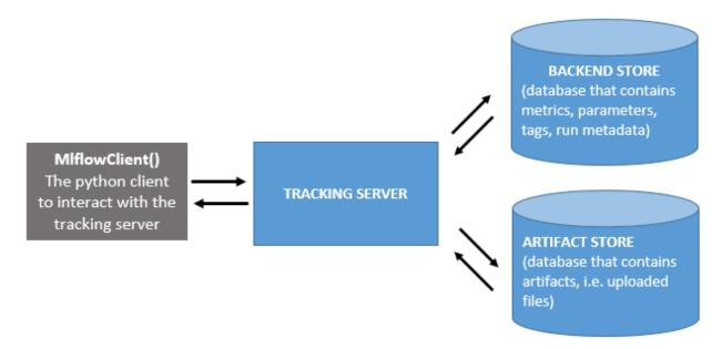
Basically, this schema shows that mlflow separates WHERE the artifacts are logged from HOW they are logged inside your code. You need to setup your mlflow tracking server separately from your code, and then each logging will send a request to the tracking server to store the elements you want to track in the appropriate location. The advantage of such a setup are numerous:
